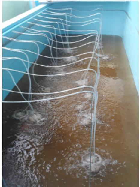
**Figure 4. Typical tank configuration in Americas — duplex, 35 m<sup>3</sup> capacity with PVC aeration pipe.**
