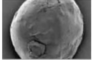
EM photograph of a microencapsulated feed
